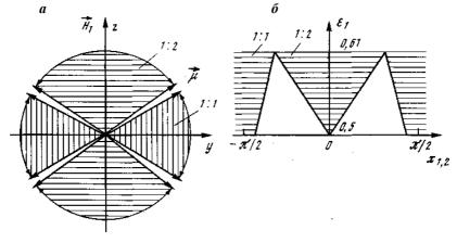
Fig. 1. Scenario for the appearance of a bifurcation for an inverted pendulum according to Poincare with  $\varepsilon_0$ =0. a) 0,5< $\varepsilon_1$ <0,61; dependency graphs of  $x_{1,2}(\varepsilon_1)$ .
