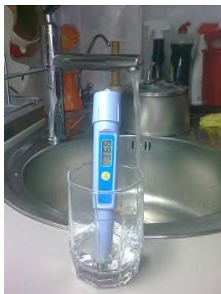
Tap water, EMF=+366 mV
